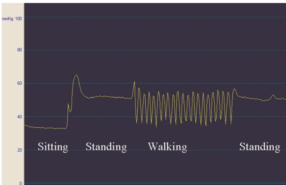
**Figure 4** Sub-bandage pressure measured by a Picopress® transducer at the medial mid-thigh level after application of an adhesive bandage. The pressure peaks during walking go up to 55 mmHg
